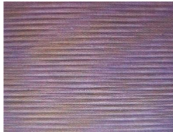
Stone ground base enlarged 100X.
